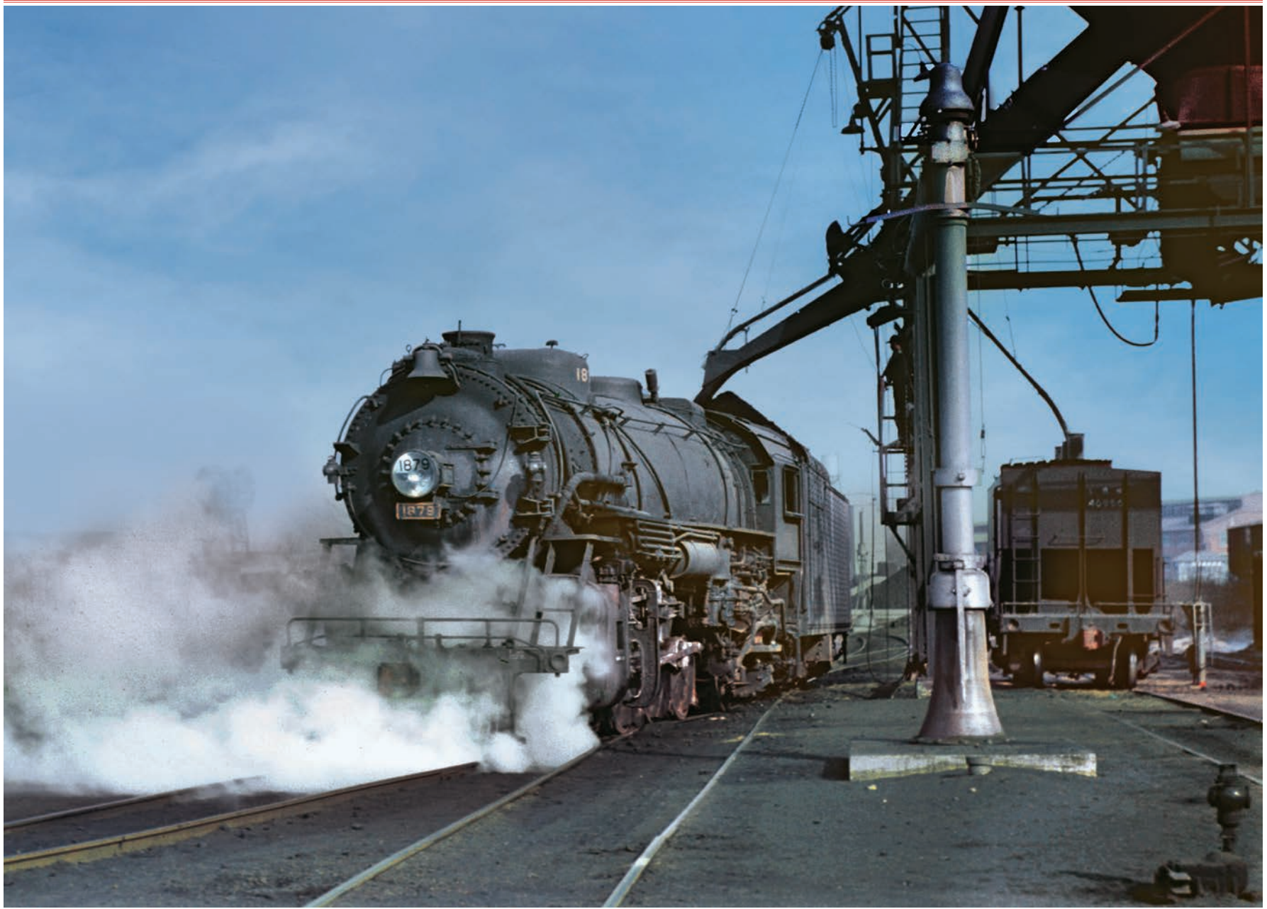
J-4 1879 was one of a few big 2-8-2s that were equipped with secondhand six-wheel-truck, high-capacity tenders purchased from C&O near the end of steam. The big tanks extended the range of the Mikes by eliminating several coal or water stops. The engine is shown in about 1951 taking coal at South Louisville. — Jack Fravert photo
